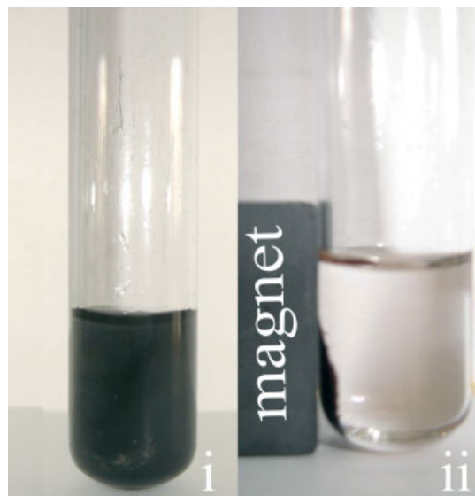
Figure 1. A reaction mixture in the absence (i) or presence of a magnetic field (ii).
